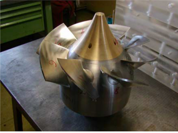
Fig. 8. Downsized model of a Deriaz pump-turbine [21].
