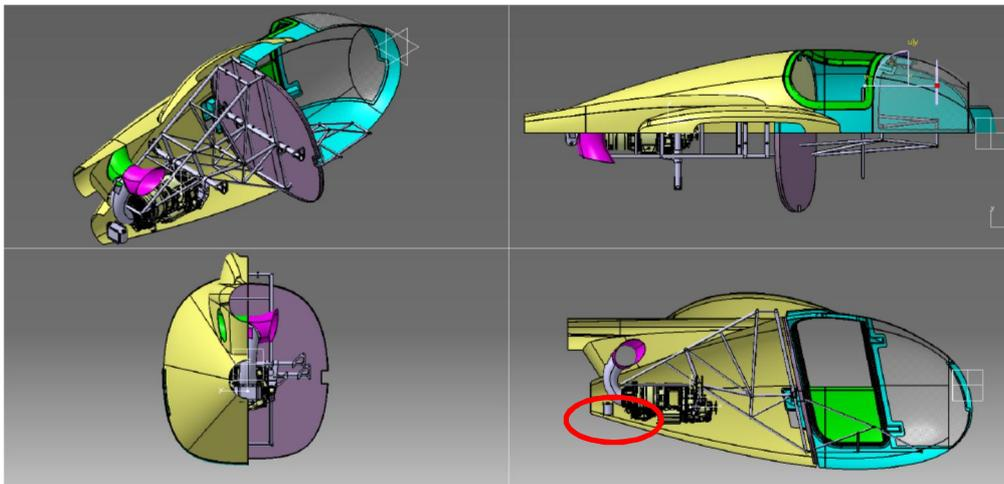
Figure 16 - 2<sup>nd</sup> heat exchanger position
