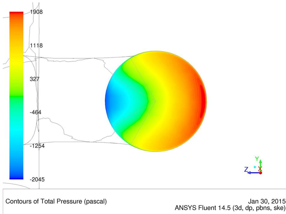
**Figure 14 – Total pressure contours at the outlet of the intake**
