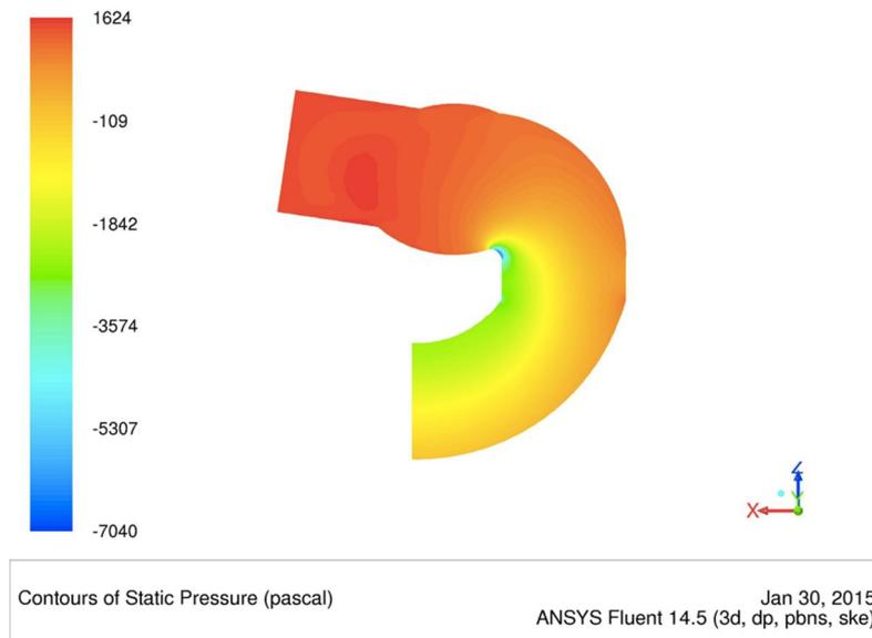
**Figure 13 – Pressure field in the air intake**
