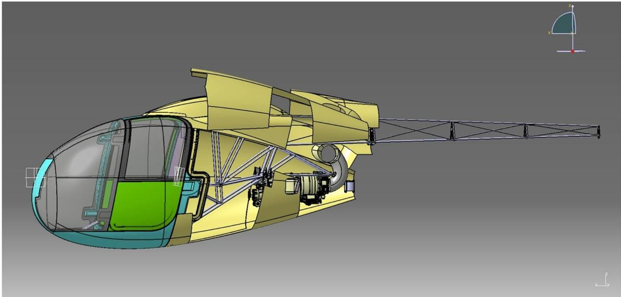
**Figure 9 – B250 engine support structure with trussed tail boom and open fuselage (with access doors)**
