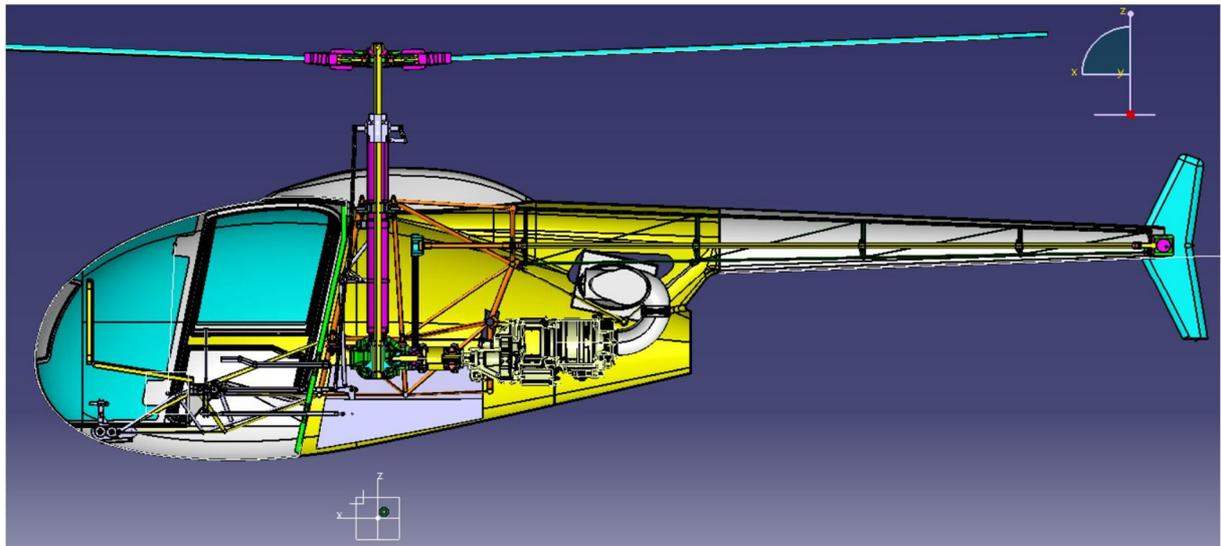
**Figure 3 - ACC HE1: TS100 in helicopter configuration on B250 aircraft – Cross section with IBF filters**
