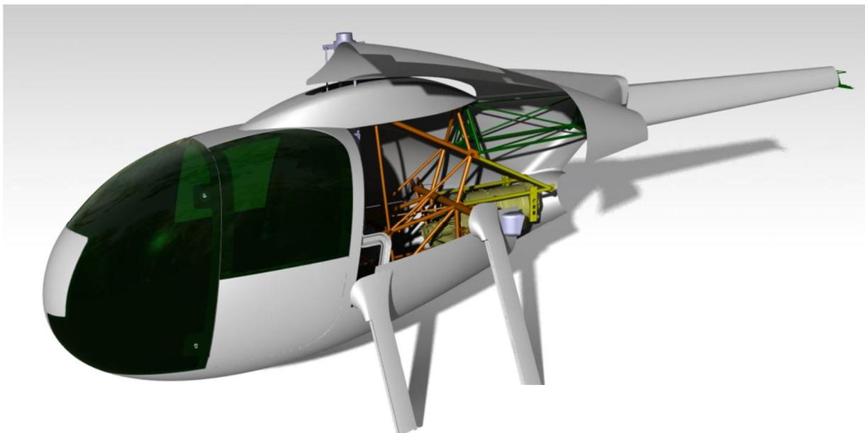
**Figure 4 – Detailed Catia view of the TS100 engine – main helicopter gearbox – chassis – fuselage B250 integration**
