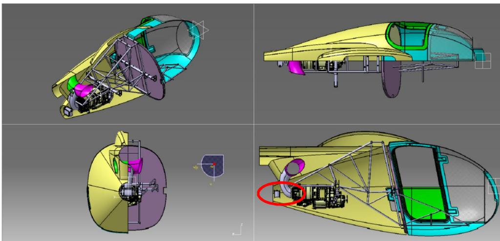
Figure 17 - 3<sup>rd</sup> heat exchanger position (best position)
