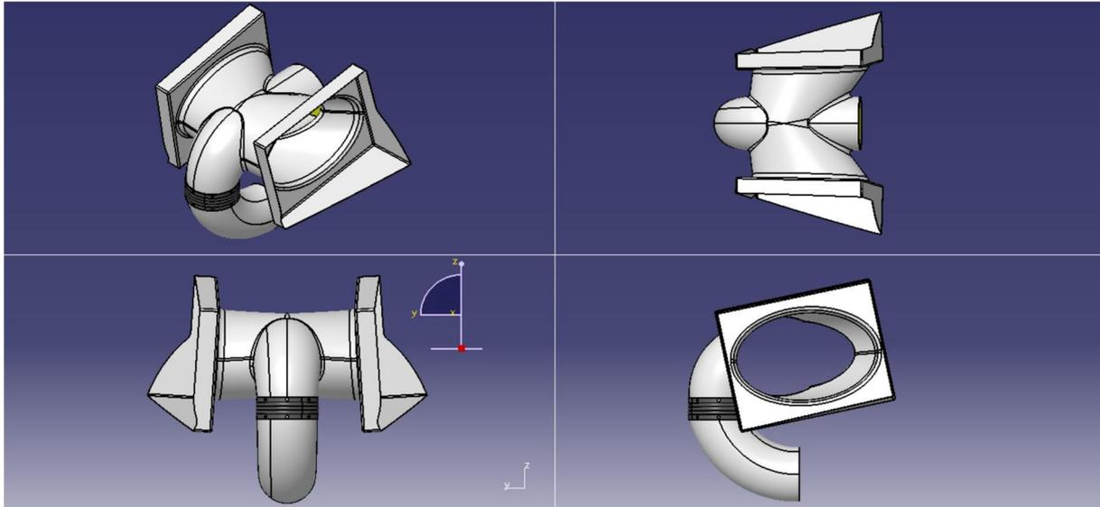
**Figure 7 – B250 air intake with IBF and by-pass door**
