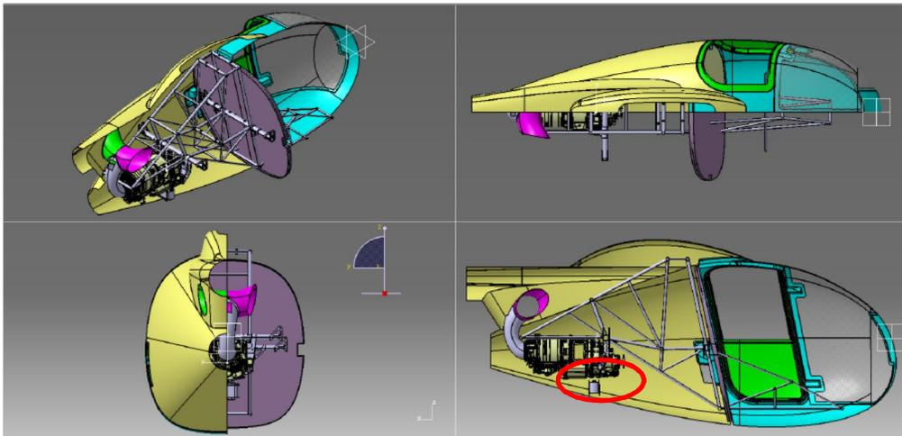
Figure 15 - 1<sup>st</sup> heat exchanger position
