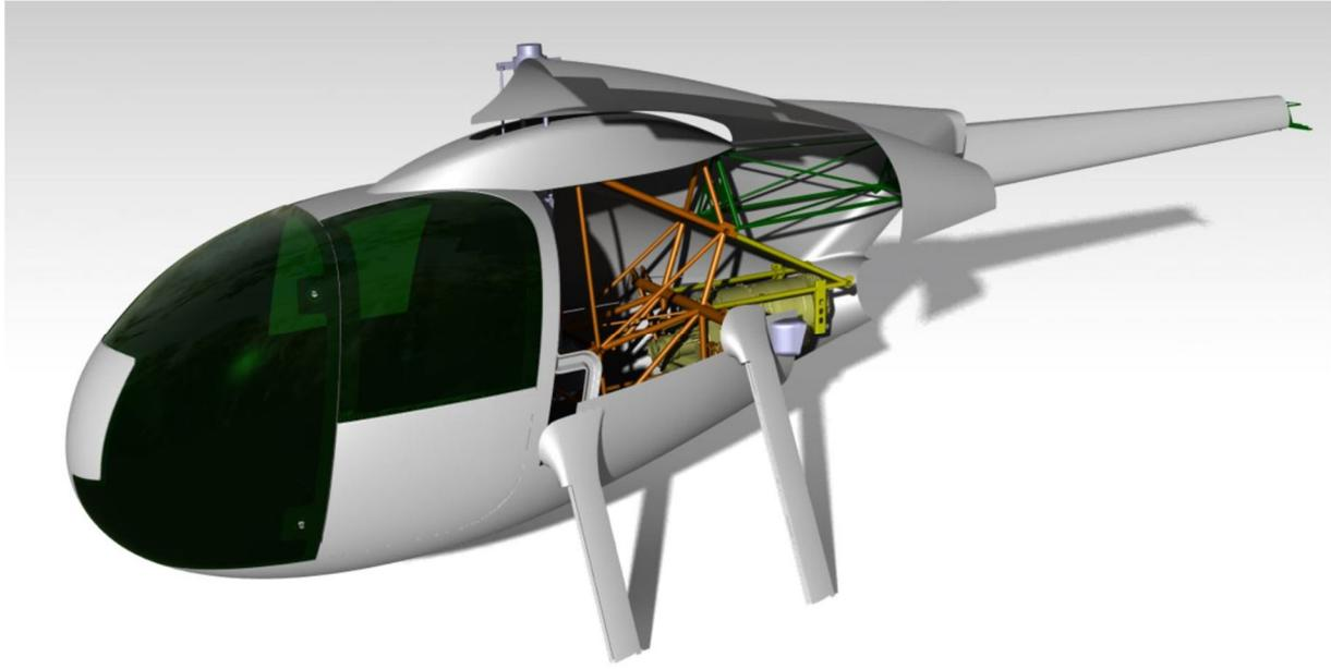
**Figure 2 - ACC HE1: TS100 in helicopter configuration on the B250 aircraft – Side view**
