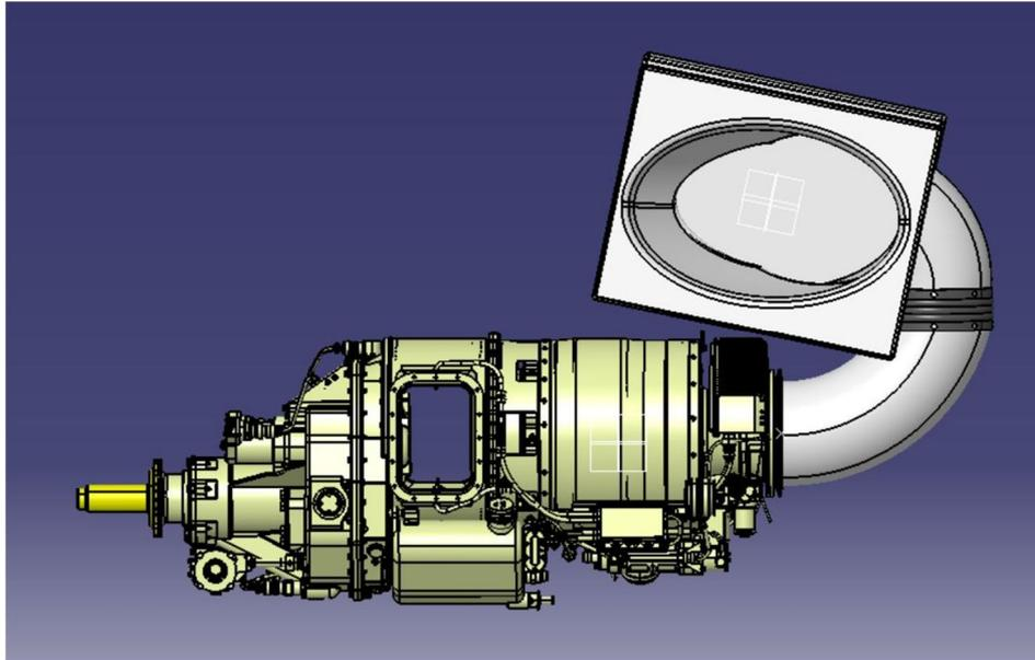
**Figure 8 – B250 air intake with IBF integrated with the TS100**
