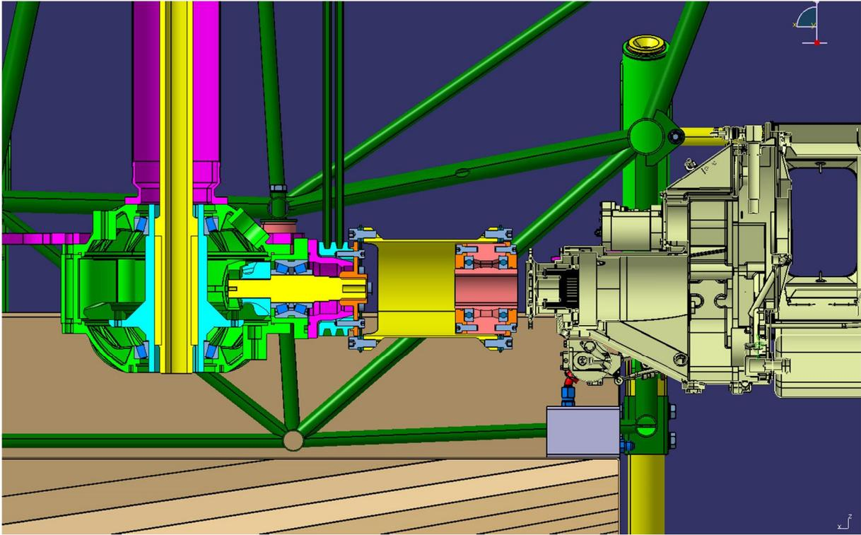
**Figure 5 – Detailed Catia view of the TS100 engine – main helicopter gearbox – chassis B250 integration**
