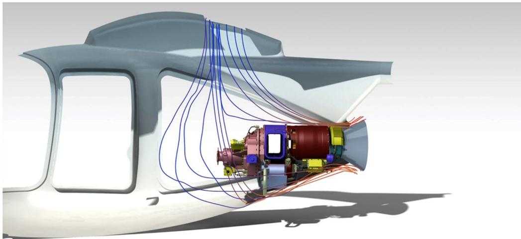
**Figure 11 - Engine nacelle ventilation – working principle (side view)**
