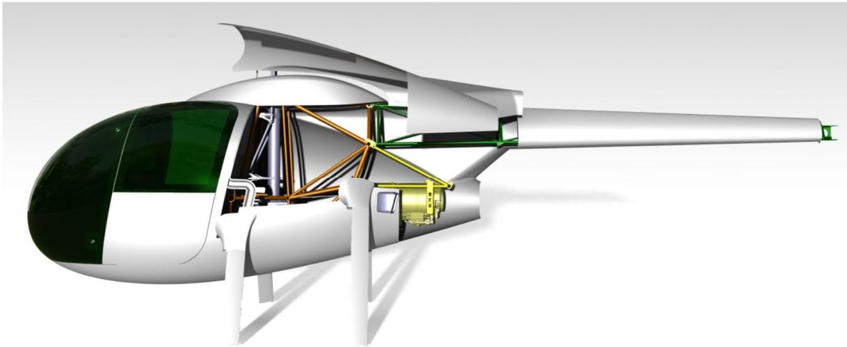
**Figure 10 – B250 engine nacelle / helicopter rear fuselage with B250 chassis**
